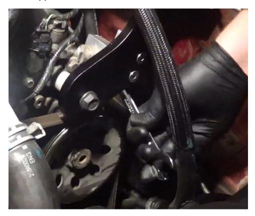
With the bolts tightened, remove the #10 bolt and discard, its job is done. Slide the #6 spacers over the #7 bolts and ready the #4 spacer and #9 bolt.
