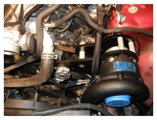
If you need to clock the Procharger, you're able to move it be loosening the 6 small allen head retaining bolts and rotating the snail like outer housing. The outlet should be pointed straight down.
