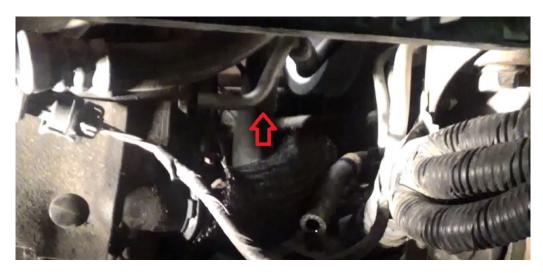
If you have a 2010-2013 model with the engine computer in the fenderwell, remove the computer from its bracket by unclipping it at the top, and follow its wiring harness to unclip and move it out of the way. You'll also want to remove the two nuts holding the bracket inplace, remove the bracket, then reinstall the nuts. Set the computer aside for now, it'll be reinstalled later with its bracket in a different location.
