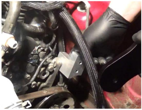
Grab the engine side mounting bracket. You'll need bolts #10, #11 and #7 and spacer #5. Identify the backside of the plate, and slide bolts #7 through the two bolts at the top of the plate so they face forward.
