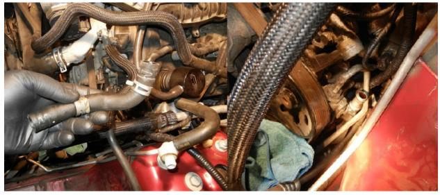
The new reservoir mounts back beside the brake fluid reservoir. The black bracket and its aluminum sub bracket goes over the stud and is secured by the same nut. The reservoir then slides down onto the black bracket. You'll need to use a little persuasion on the A/C line to give the reservoir some clearance.
