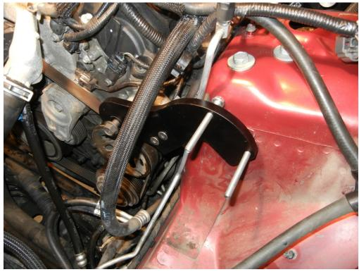
Using bolt #10 and spacer #5, slide the bolt through plate from the front side, then through the spacer, and attach to the existing threaded hole on the front of the engine, hand tighten the bolt. Rotate the plate until the countersunk holes and the threads in the #3 bracket line up, and use the #11 bolts to secure. Tighten the #10 bolt snug to line up the plate, then torque the #11 bolts to 15ft-lbs to connect the two brackets.
