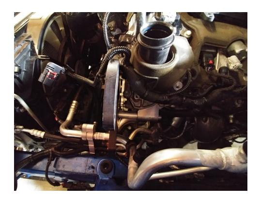
Use spacers #1 and #2, and bolts #2 and #4 to put the plates together; the thinner bolts and spacers go to the top of the plates and come through the backside, and the larger diameter closer to the tensioner goes through the front side. Torque screw #2 torque to 35 ft-lbs and #4 screws to 18 ft-lbs.
