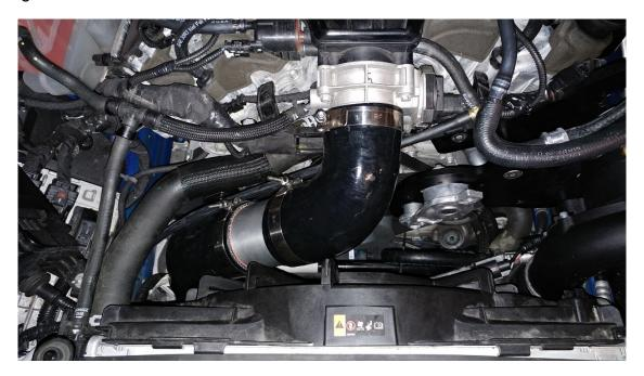
Now is a good time if you've not done so yet to take the ¼" hose from the BOV throttle body spacer kit and run it from the spacer to the BOV vacuum fitting on its top.
