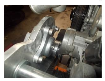
**Step 8: Install Mounting Plates and Supercharger**
