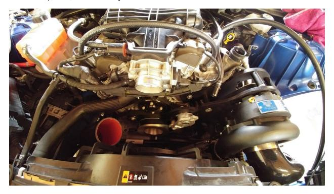
Step 9: Installing the Intercooler
