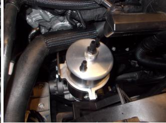
The bracket, a long L bracket will bolt to the 15mm headed bolt on the front of the engine cover behind and below the radiator hose as shown. Make sure the L portion faces toward the left side of the engine compartment with the cutaway up:
