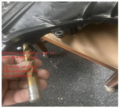
All lines tuck in so the engine cover installs back as stock, and only the
