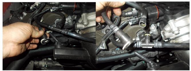
Above you will un-clip the cleanside line from the muffler and then carefully slit the end on the T and remove. Save this if you need to put back to stock in the future. Unclip both fittings of this tube that bridges each valve cover and using a large screw driver carefully pry up each barb from the valve cover. Drill with a 1/4" drill bit through so they flow without restriction, and clean and reseat back into the valve covers. Then reclip the hard line back onto each.
