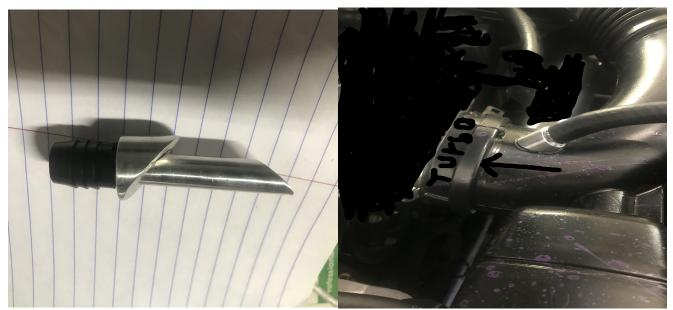
The second outer fitting from the can with inline checkvalve flowing AWAY from the can will connect to this barb. It does not need to be super close to the turbo, just between the cleanside barb and the turbo. Seal with RTV and tape or zip tie in place until RTV cures overnight.
