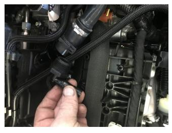
Now run this directly to the last outer fitting on the can (either side will work) with inline checkvalve flowing AWAY from the can. This will provide evacuation when in boost where when stock there was only evacuation at idle and deceleration. Now contaminants are being removed all of the time. The full time evacuation keeps your oil cleaner longer, and extends your engine life.
