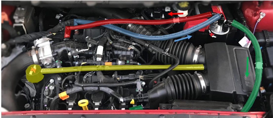
Figure 8: Plumbing Diagram Foul Side (Blue), Intake Vacuum (Red), Turbo Inlet (Green), and Clean Side (Yellow)
