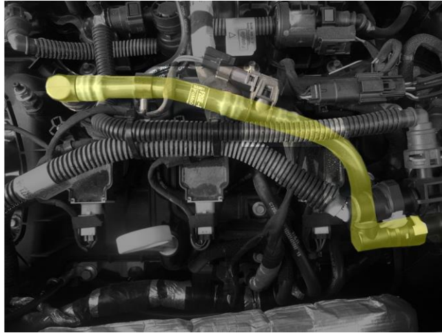
Figure 3: Line connecting clean side port to turbo inlet port to be removed.
