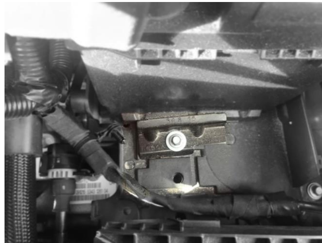
Figure 4: Battery tie down and hole to be drilled out
