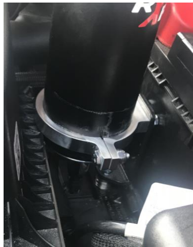
Figure 7: Placement of Catch Can and Clamp
