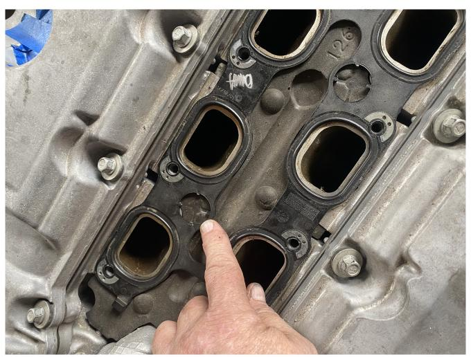
On the stock gasket, snip the 4 legs and remove the round hump.
