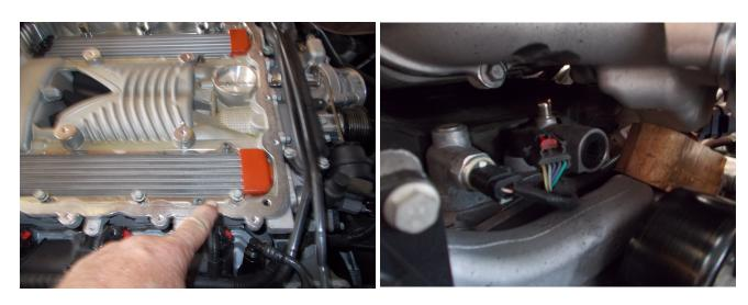
As you can see above simply prop up the blower with a small piece of 2x4 or similar. The PCV valve has a large allen socket and unscrews: Remove the 2 O rings from this and install them on the billet diverter unit and screw it into place just snug:
