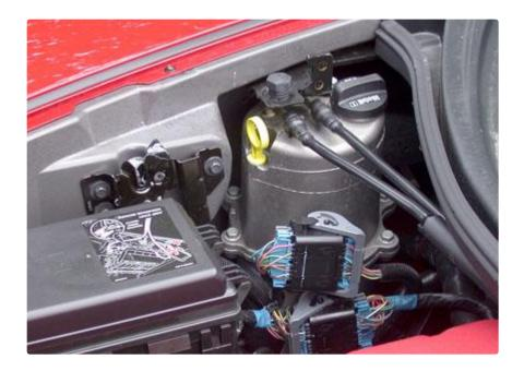
The clean side separator will replace the oil fill cap on the dry sump oil tank. The bottom plastic portion slips off and installs just as your stock oil cap, and the main separation unit then pushes into it sealing with dual O-rings.
