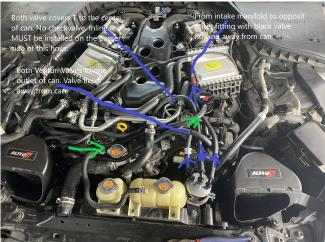
You may need to relocate the fan controller so the can can mount as shown:
